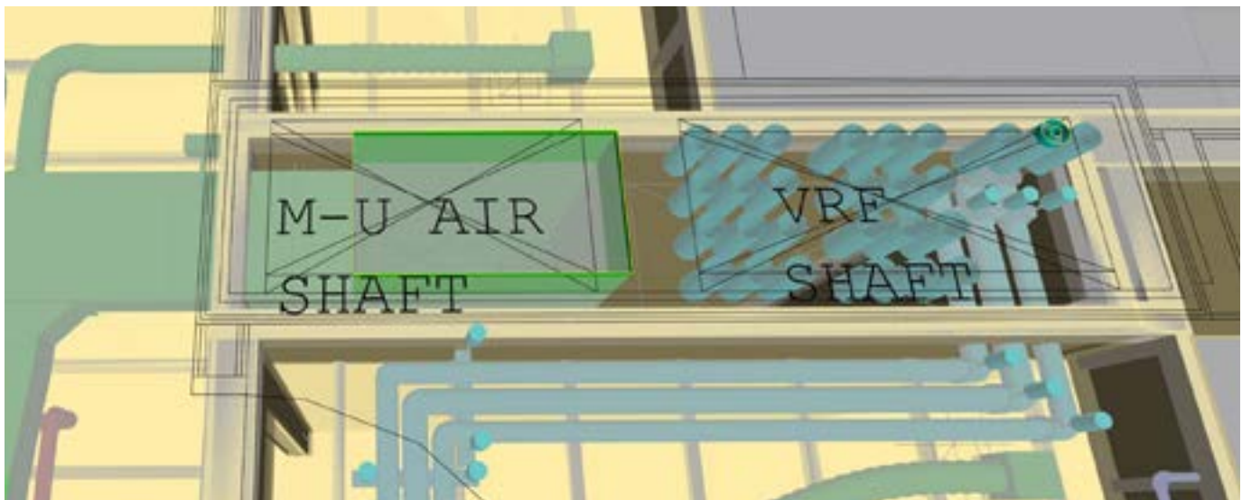
Figure B.2.3. This image shows a M-U air shaft and VRF shaft designed in BIM. The original architectural and structural plans had designed the shaft size to encompass both the M-U duct and VRF piping. However, the detailer was able to create a separate shaft.
