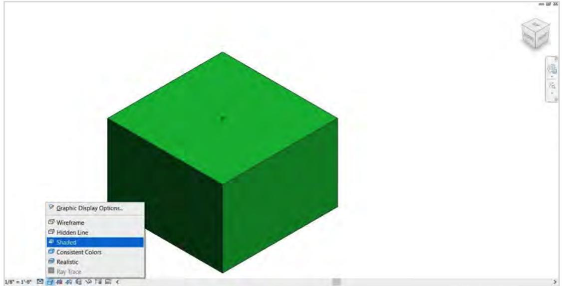
Figure 63 – Choose Default 3D View and apply Shaded visual style to see the color of the geometry.
