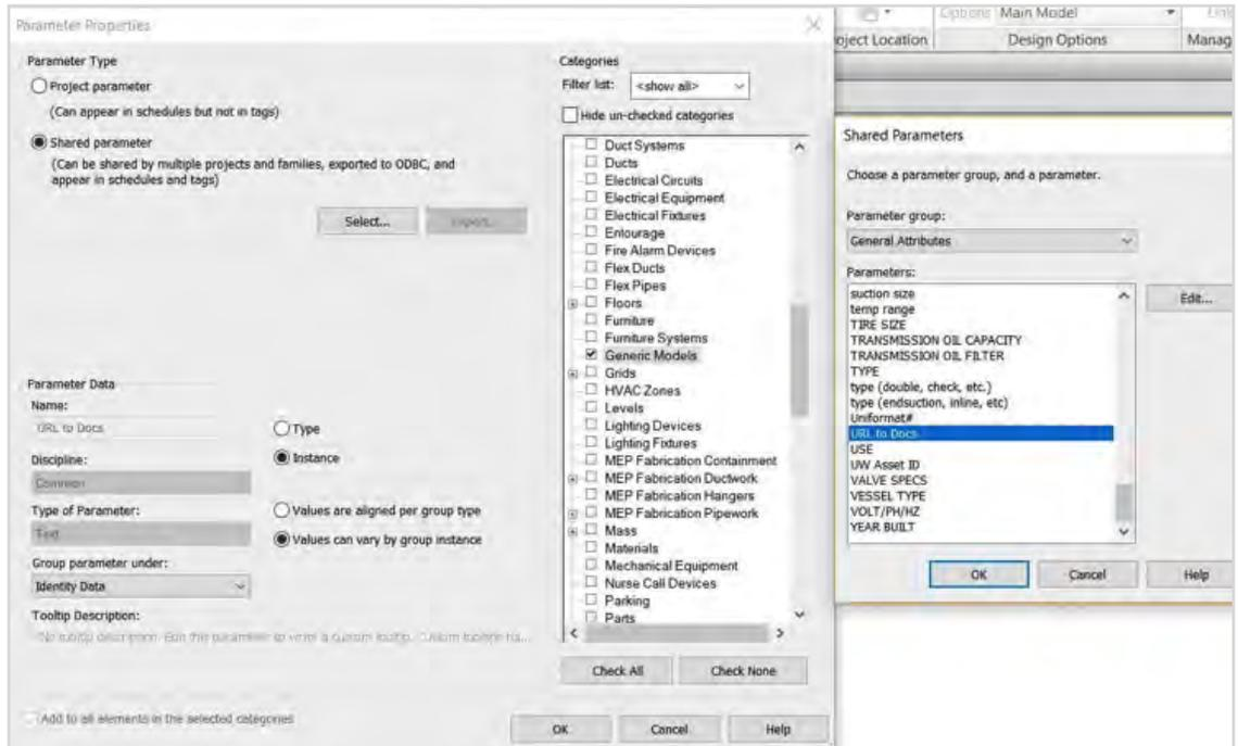
Figure 80 – Adjust settings in Parameter Properties and add attributes from Shared Parameters.
