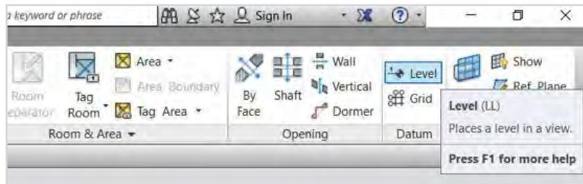
Figure 85 – Use Level command from the Architecture tab to add to building levels.
