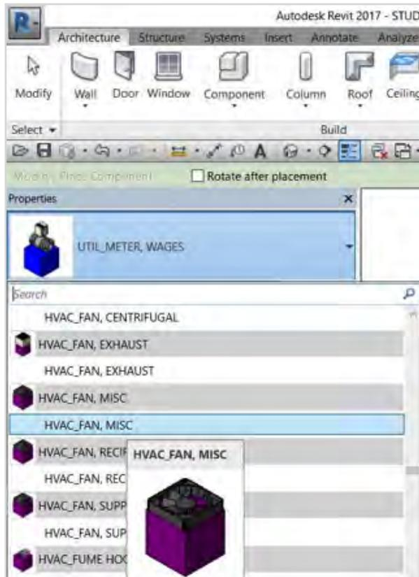
Figure 78 – Accessing the asset families from the Properties window (after enabling the Architecture tab and Component command).
