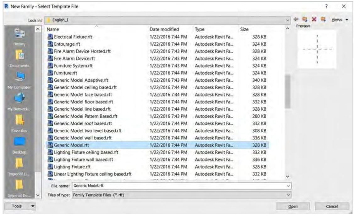
Figure 35 – Open Generic Model.rft as the required family template.
