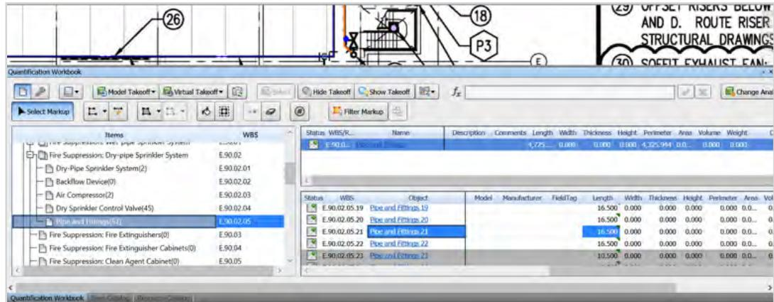
Figure 26- Overriding the length parameter for a riser.
