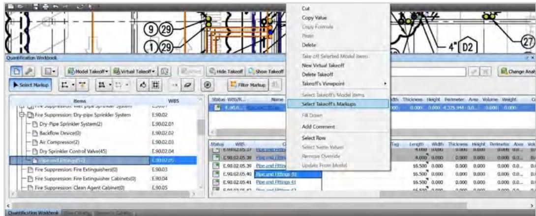
Figure 27- Finding asset mark-ups by selecting data fields.
