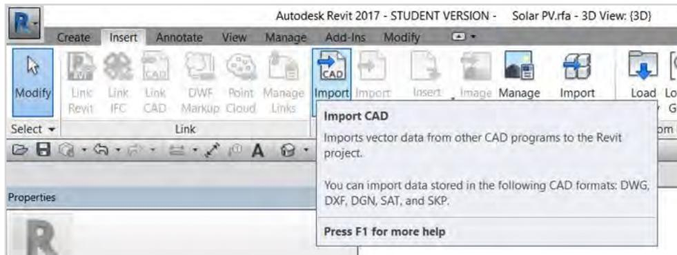
Figure 69 – Import CAD geometry into Revit family.
