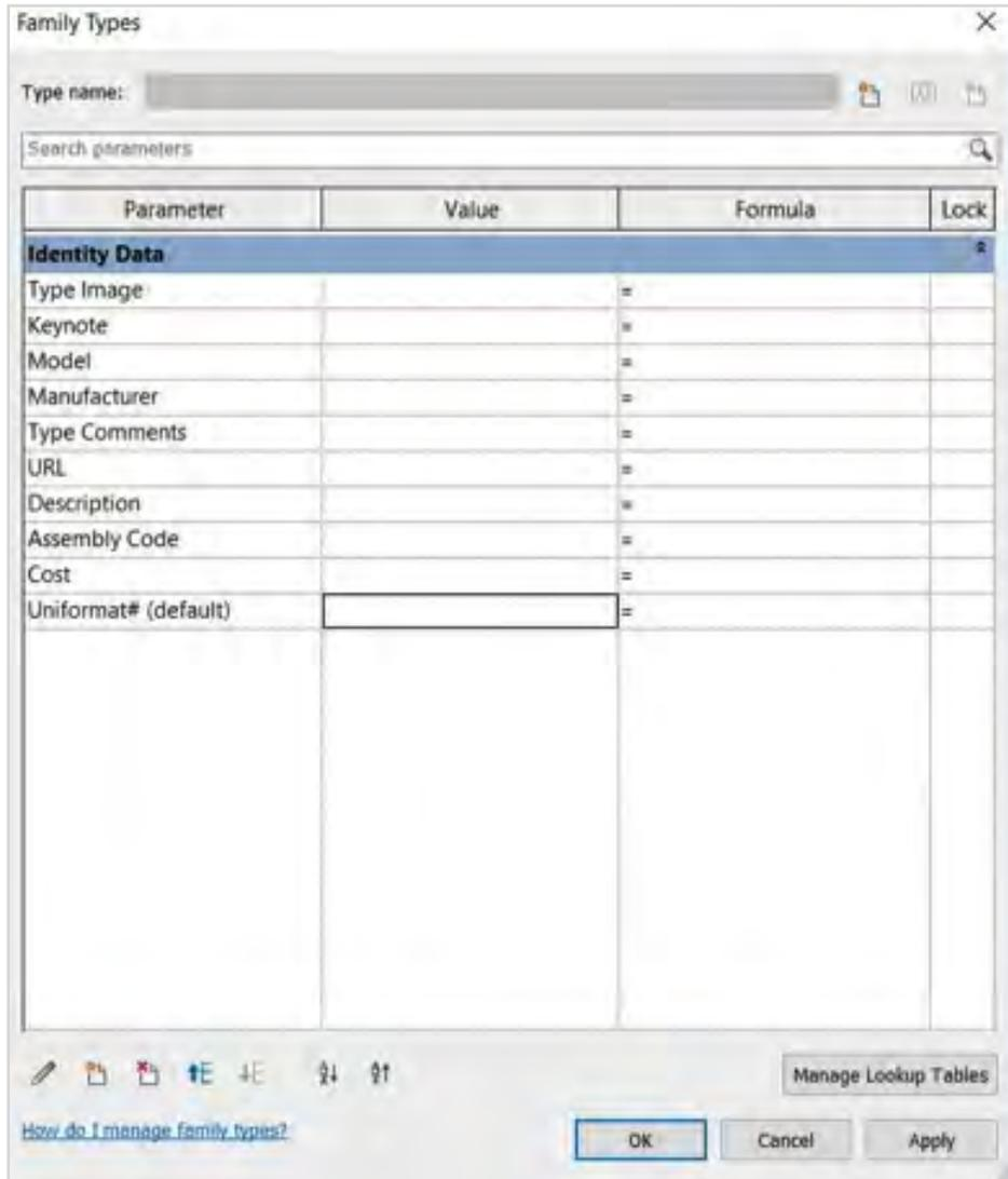
Figure 55 – The parameter added is to the identity data attributes of the family.
