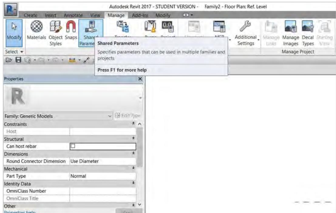
Figure 36 – In the Family Editor Environment, from the Manage tab, open Shared Parameters.
