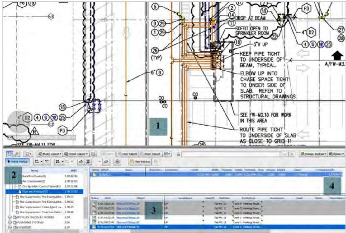
Figure 25 – 1: Mark-ups on drawings; 2: Asset categories; 3: Asset instances and attributes in data worksheet; 4: Total quantity for the selected asset category.
