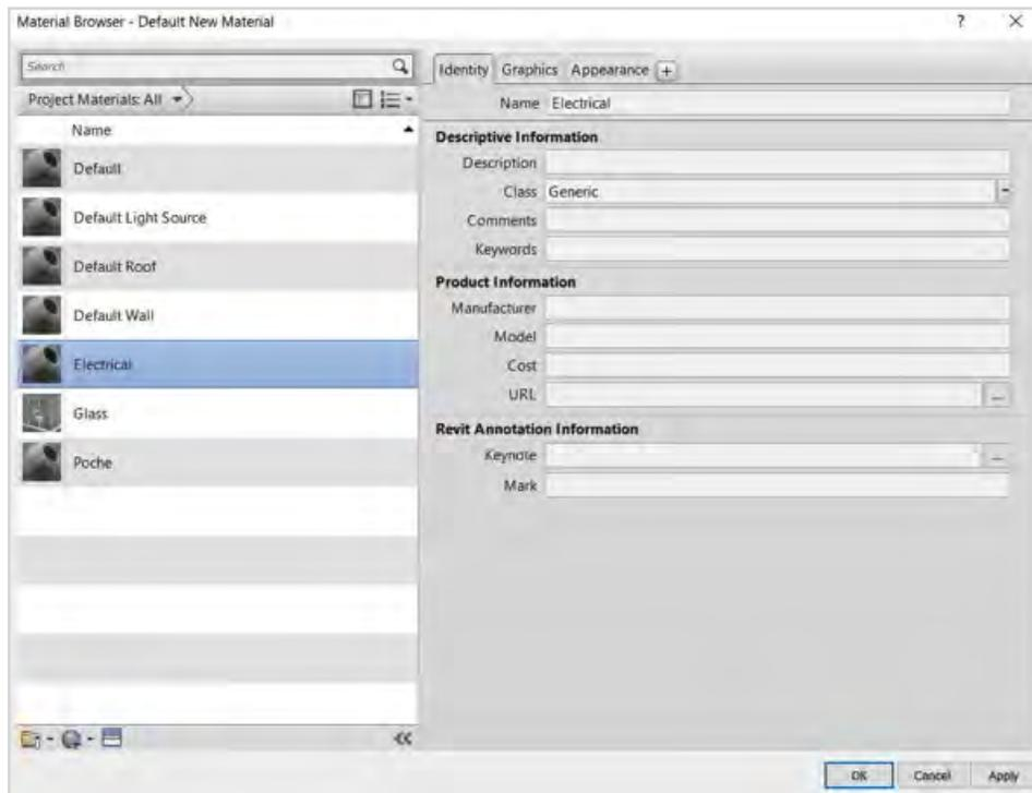
Figure 60 – Rename the material in Identity tab.
