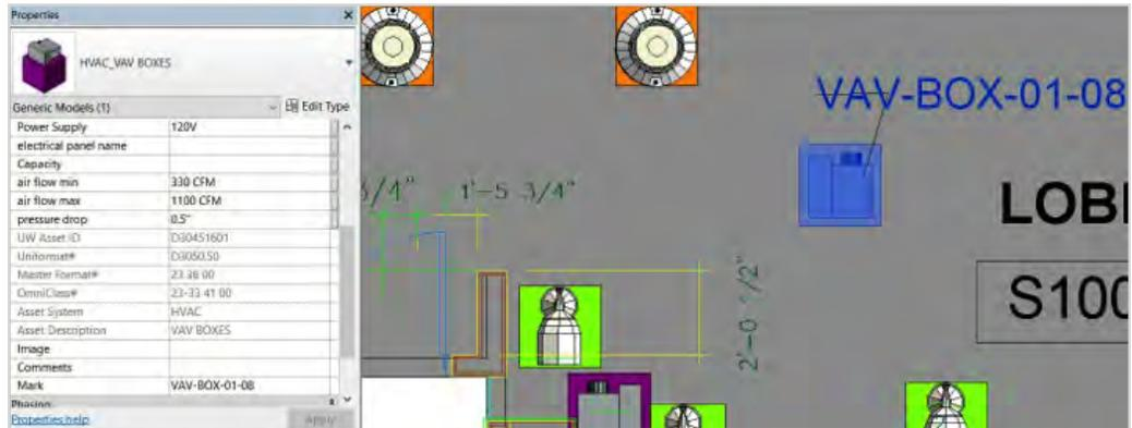
Figure 89 – Filling in attribute fields of each asset instance in the Properties window.
