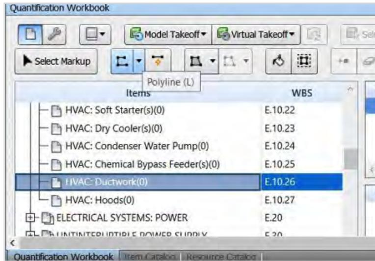
Figure 23 – Selecting an asset category (HVAC Ductwork) and the relevant mark-up tool (polyline).
