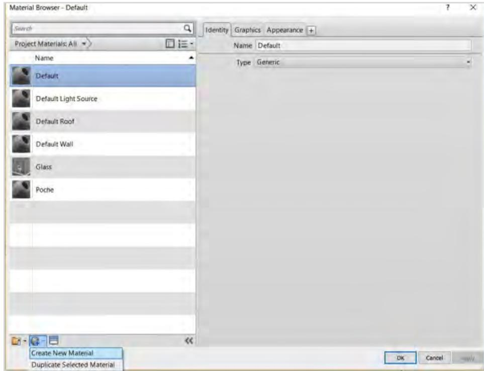
Figure 59 – Create a New Material from the lower toolbar.
