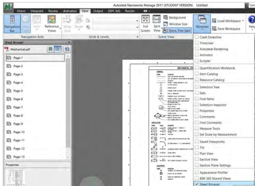
Figure 13 – Enabling Sheet Browser window in Navisworks interface.
