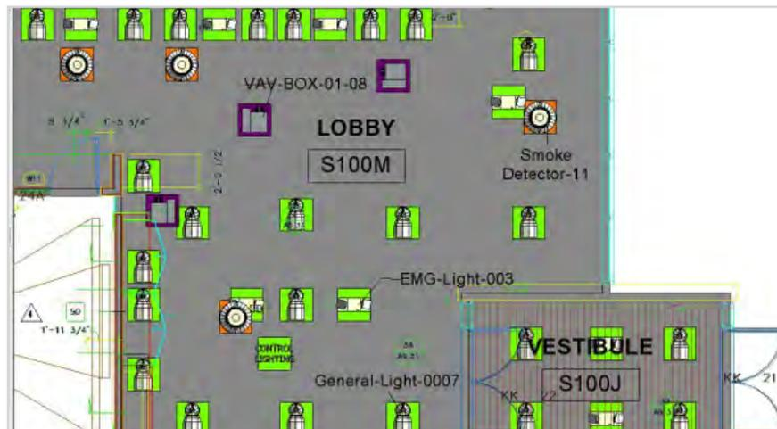
Figure 88 – Example for placing multiple asset instances on a drawing.
