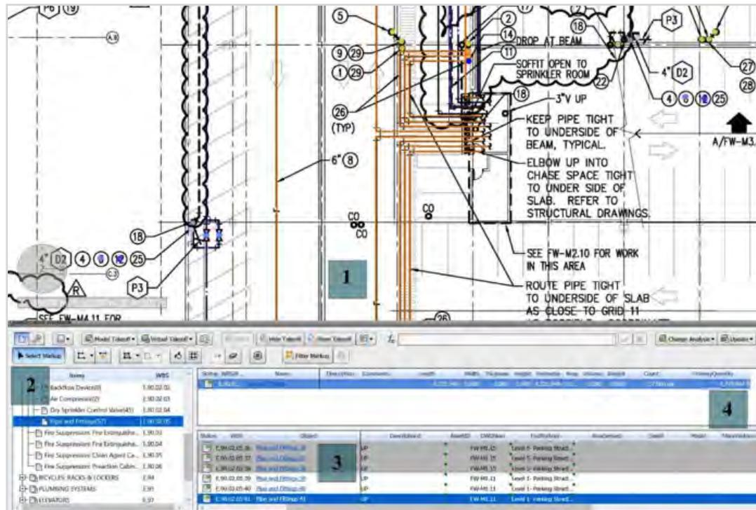
Figure 1 – User interface in Navisworks for rebaselining. 1: Mark-ups on drawings; 2: Asset categories; 3: Asset instances and attributes in data worksheet; 4: Total quantity for the selected asset category.
