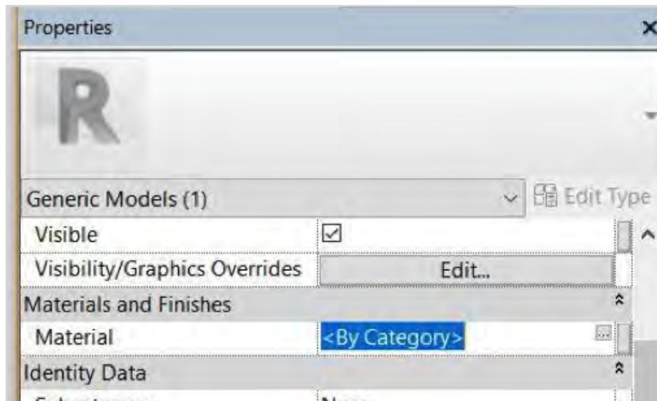
Figure 62 – Assign the material to the box.
