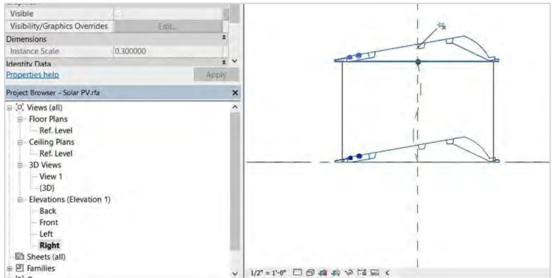
Figure 72 – Use Right Elevation to position the imported geometry.
