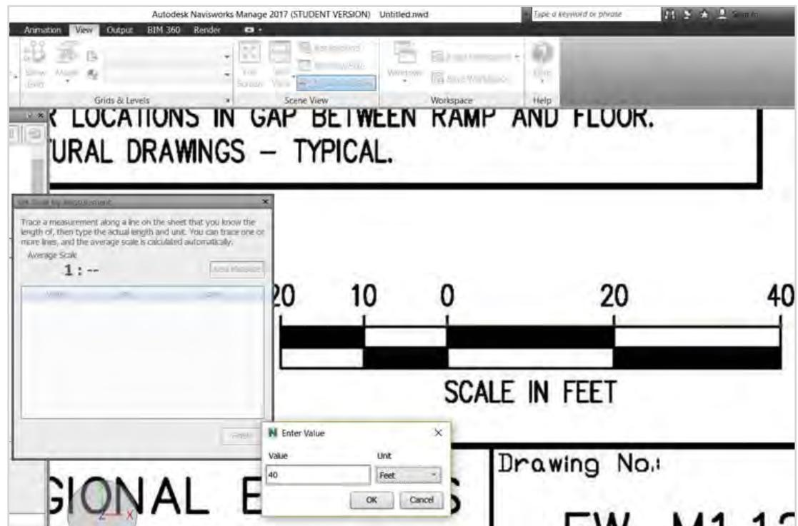
Figure 20 – Set scale of drawings by measurement (a line is drawn from 0 to 40 and its length is specified in Enter Value window).
