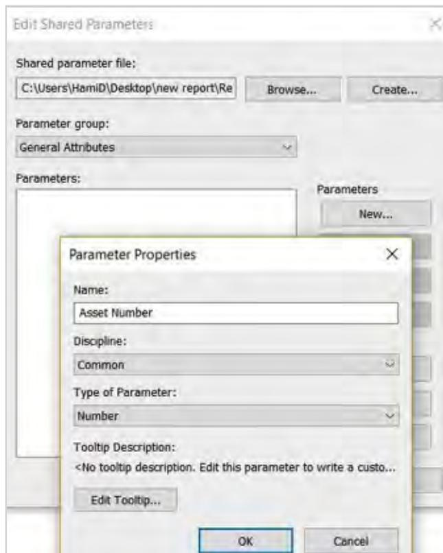
Figure 41 – Set the name, discipline, and type of parameters.
