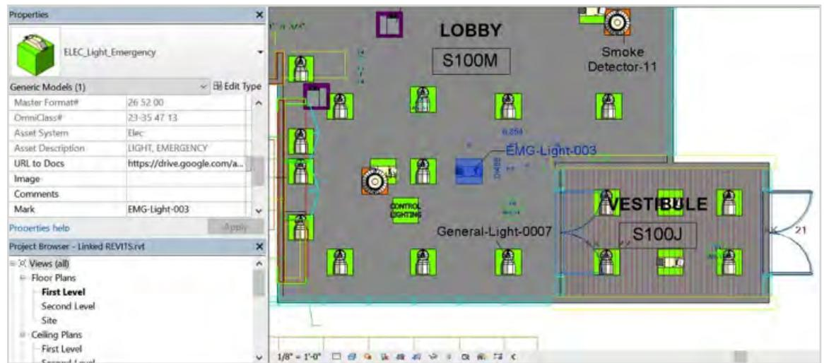
Figure 4 – Asset data model created in Revit (asset instances + data attributes).
