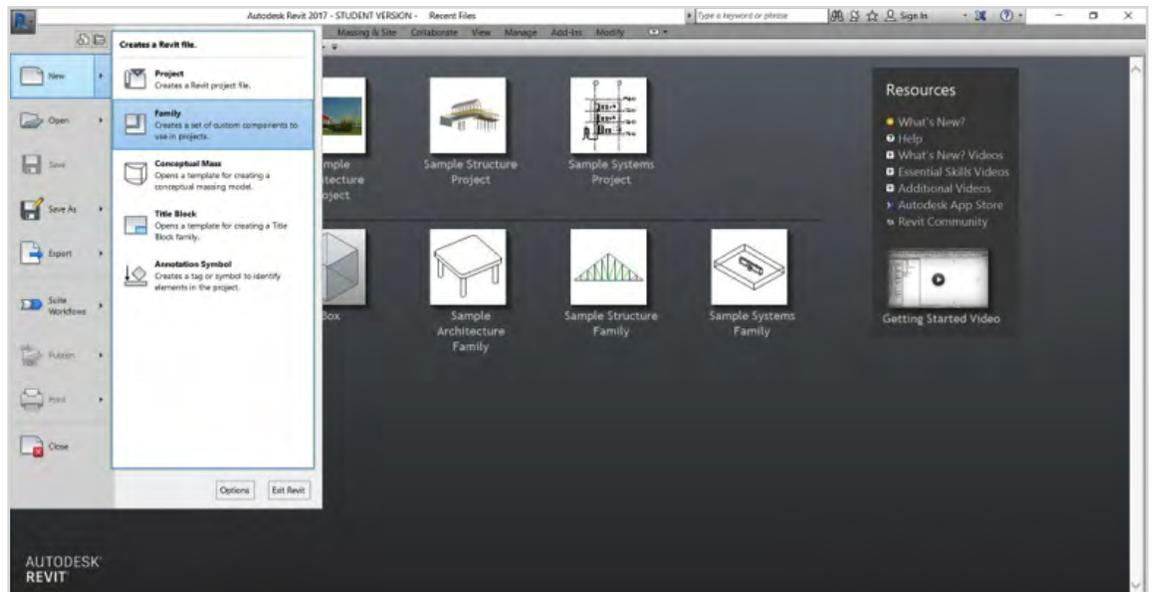
Figure 34 – Open Revit and create a new family.
